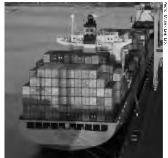
Typical containership with container-carrying holds between the deckhouse and bow, and space for additional containers to be stacked aft of the deckhouse.
